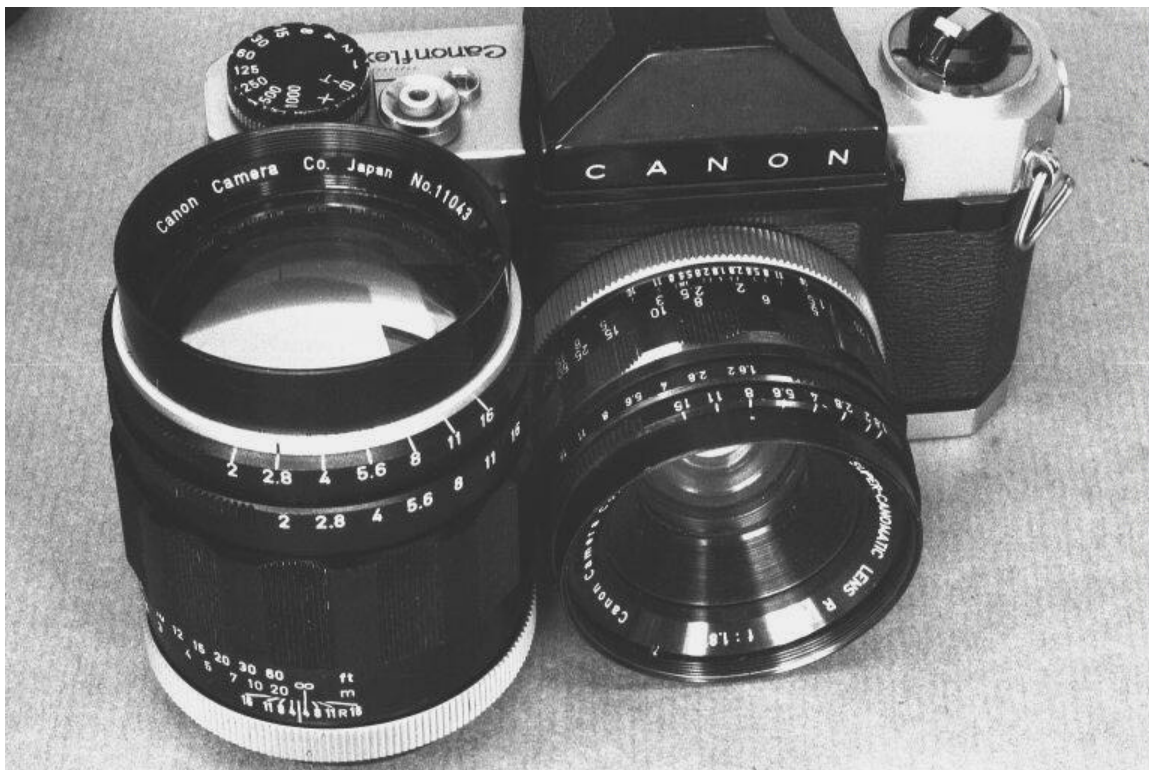
Fig 033 034 Canonflex lenses with stripes at iris setting.
