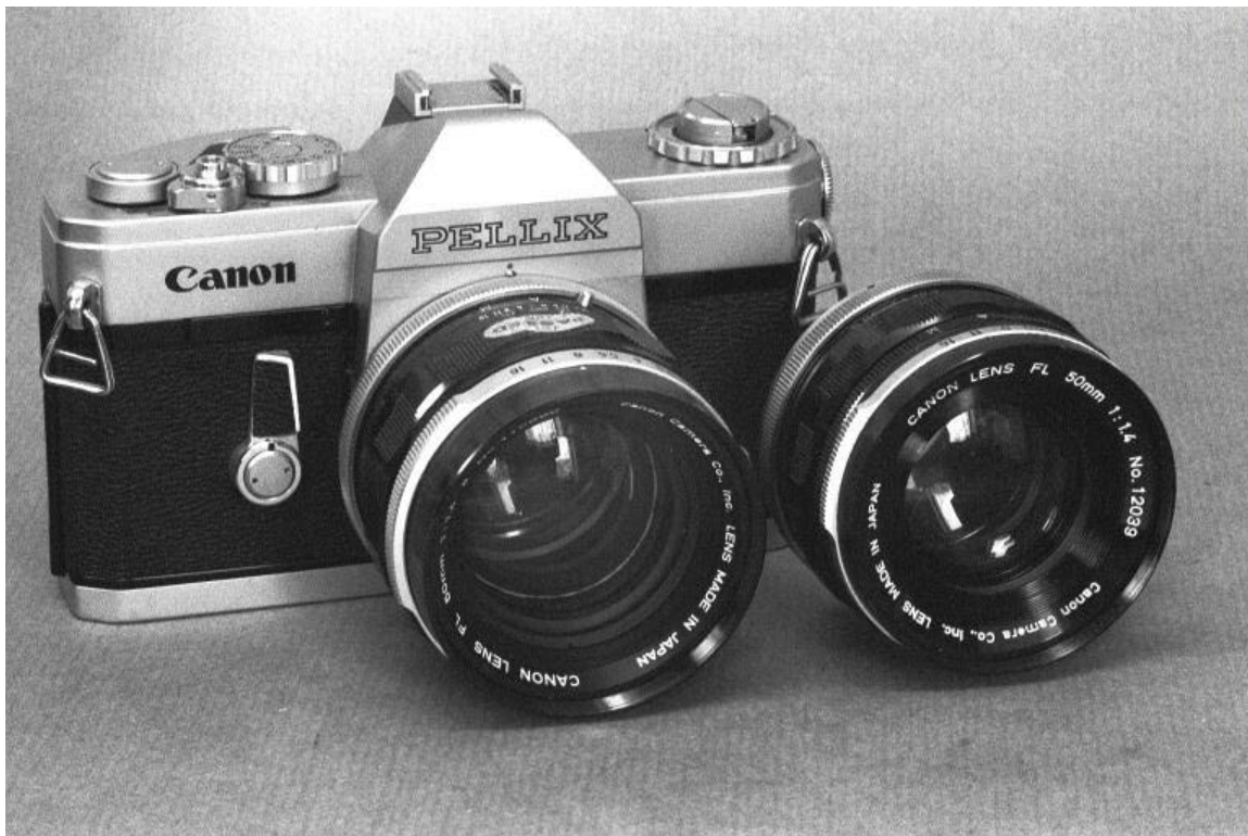
Fig 033 012 Canon Pellix with 2x Canon f1.4/50mm lenses.
