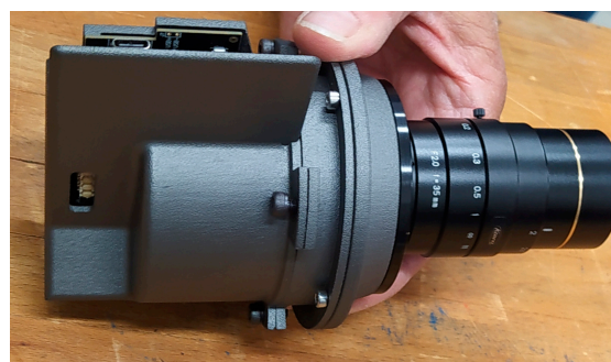
Figure 8. One of the STARLITE current shelves realized with 3D printing, mounting the Kowa 35 mm objective LM35XC by Kowa Optimized, Deutschland GmbH (Duesseldorf, Germany). STARLITE supports standard C-mount optics, enabling flexible FOV adjustment via interchangeable objectives.
