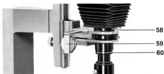
Fig. 21a Synchronized time- and instantaneous shutter 58 bellows locking lever 59 tape measure 60 marking on the lower light screening collar
