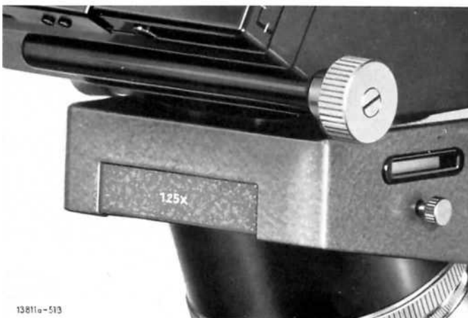
Fig. 12 Revolving nosepiece with tube factor engraved
