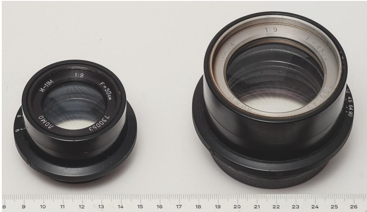
Fig. 14: Two of the older “Industar 11M” process lenses from the USSR, made by LOMO. They are Apo-Tessar-type lenses. Left: a 300mm f/9 from 1973; Right: a 450mm f/9 from 1970. Scale is in cm.
