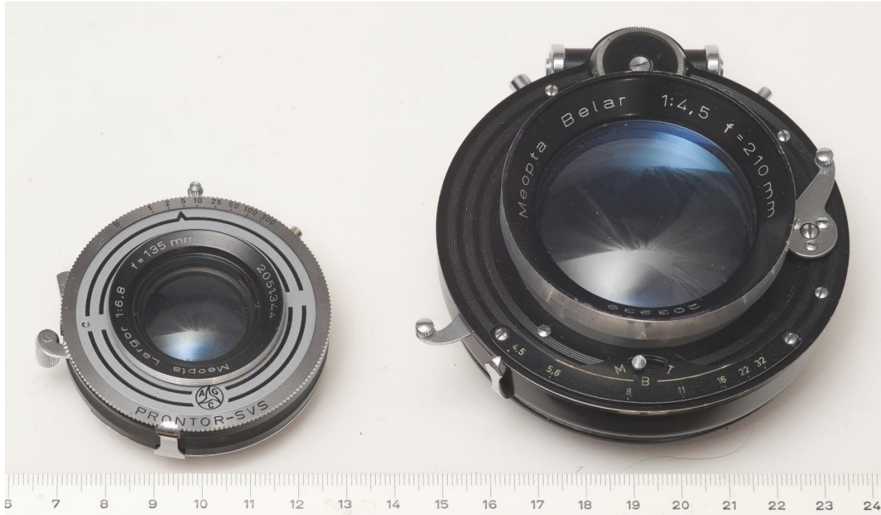
Fig. 6: Shuttered LF lenses made by Meopta for the “Magnola” technical camera. Left: Largar 135mm f/6.8 in Prontor-SVS 0, a 4/4 double Gauss wide angle. Right: Belar 210mm f/4.5 in Compound III, a Tessar type lens. Scale is in cm.
