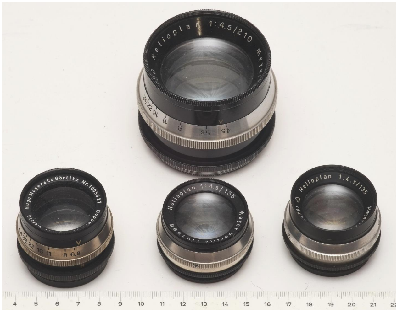
Fig. 4: Front row from left to right: Doppel-Anastigmat 210mm f/6.8 , Helioplan 135mm f/4.5 from 1949, Helioplan 135mm f/4.5 from 1954. Note the different barrel styles of the two Helioplane. Back row: Helioplan 210mm f/4.5 . The Helioplan lenses, a Dialyte construction, were sold as enlarging lenses. All lenses are uncoated, including the 1954 version. Scale is in cm.
