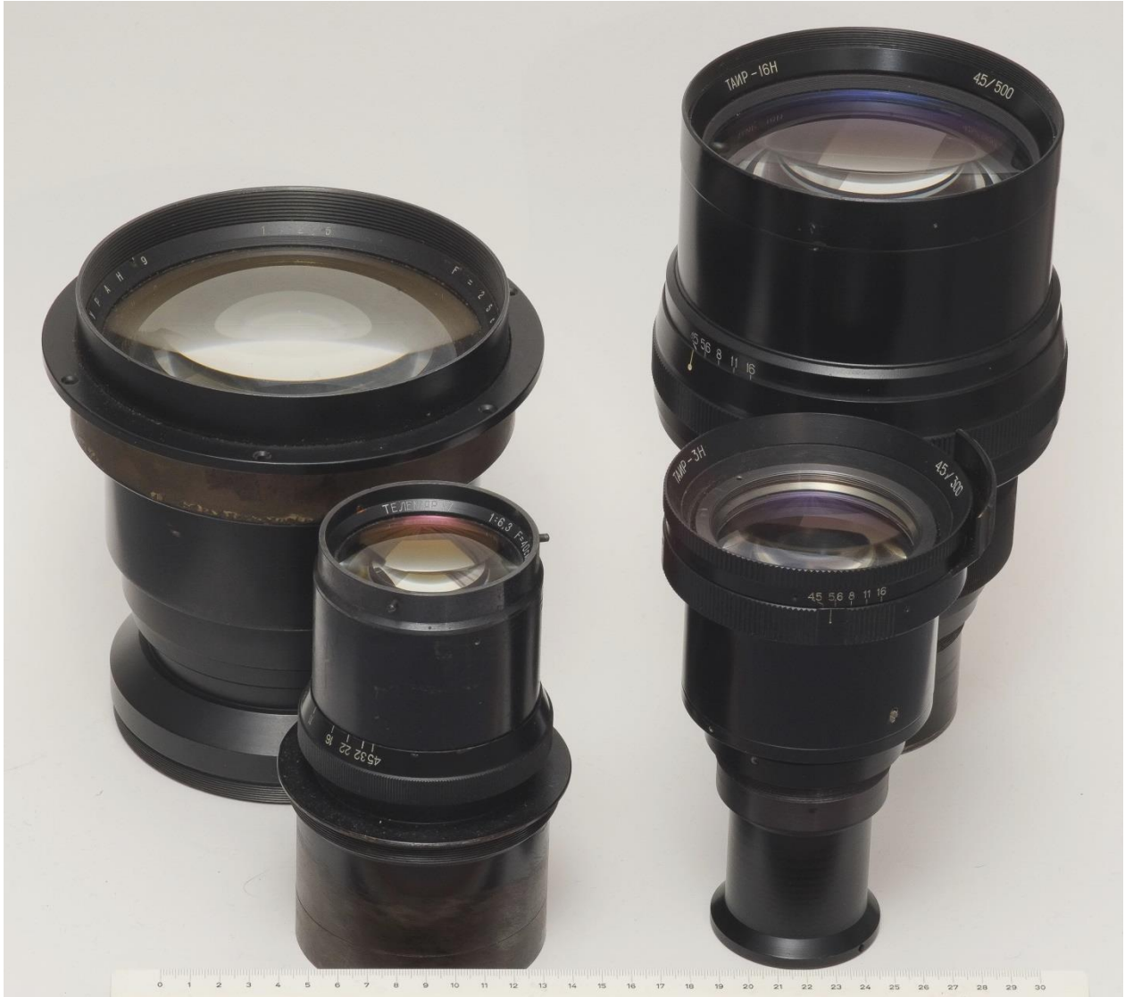
Fig. 16: Aerial surveillance lenses from the USSR. Front row from left to right: “Telemar-17” 400mm f/6.3 made by KMZ and “Tair-3N” 300mm f/4.5 (the image circle of this lens is too small for LF, it was probably used for medium format). Back row from left to right: “Uran-9” 250mm f/2.5 made by KOMZ in 1964 and “Tair 16N” 500mm f/4.5, with the official coverage similar to the 300mm. The two “Tair” lenses came as a set in a box and were made in 1977. Scale is in cm.
