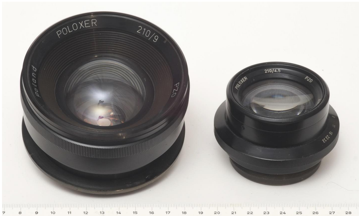
Fig. 8: Large format and process lenses from PZO. Left: Poloxer 210mm f/9 process lens, a wide angle Topogon type similar to a Process Nikkor or G-Claron WA lens. Right: Poloxer 210mm f/4.5, a Tessar-type lens. Scale is in cm.
