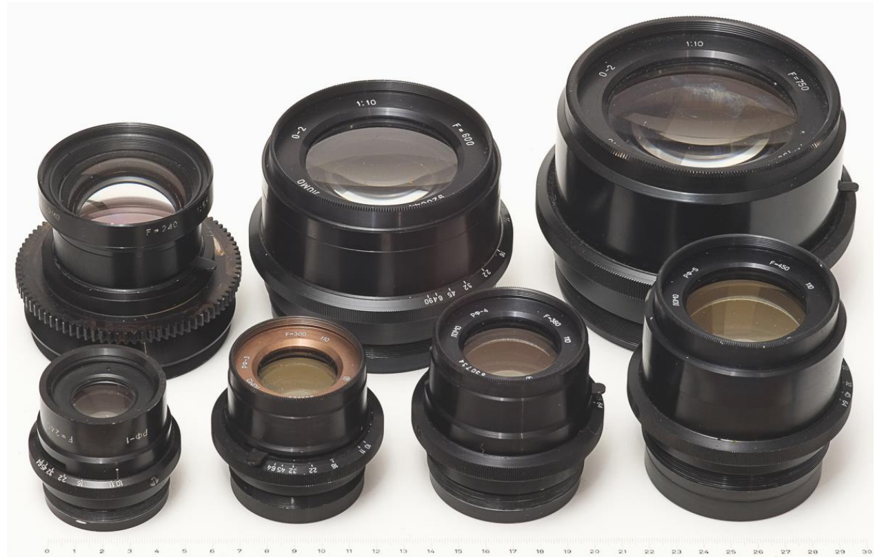
Fig. 15: Process lenses from the USSR. Front row from left to right: “RF-1” 240mm f/10 (1990), “RF-3” 300mm f/10 (1986), “RF-4” 360mm f/10 (1983), and “RF-5” 450mm f/10 (1987), all 6/4 Planar type lenses with a coverage of 45°. Back row from left to right: “RF-240” 240mm f/5.6 Plasmatic-type lens from 1987; “O-2” 600mm f/10 (1992) and “O-2” 750mm f/10 (1973), both 4/4 Dialyte-type lenses. Scale is in cm.
