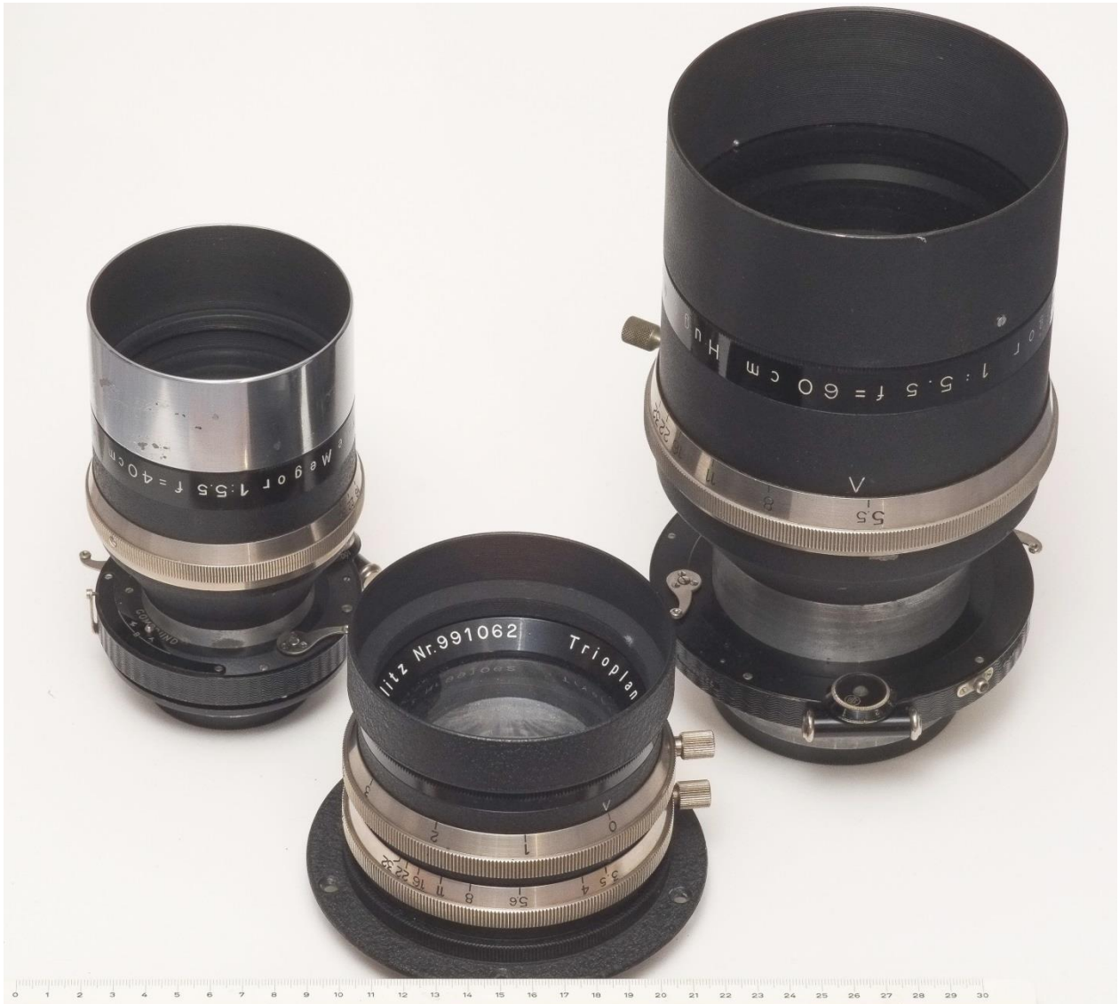
Fig. 3: Front: Trioplan 260mm f/3.5 with adjustable soft focus setting; the adjustment (upper nickel plated ring with numbers from 0-3) moves the negative center lens. Back row from left to right: Telemegor 400mm f/5.5 in Compound III, Telemegor 600mm f/5.5 in Compound V. Note that in both Telemegors the aperture is set by the nickel-plated ring of the front barrel, not by the shutter. The lenses are uncoated and were probably made during WWII. Scale is in cm.
