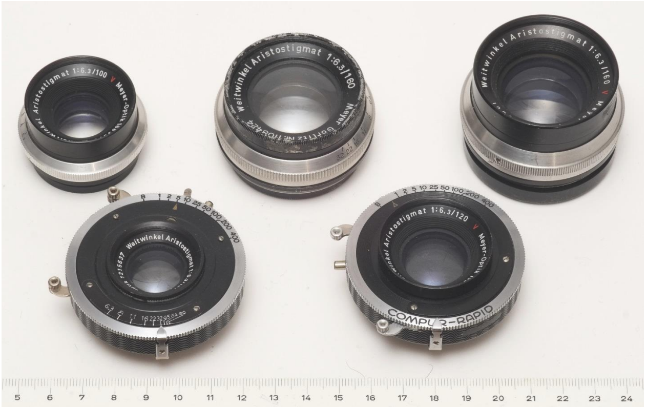
Fig. 2: Post-WWII “Weitwinkel Aristostigmat” wide angle lenses from Meyer-Optik. Bottom row from left to right: coated 100mm f/6.3 in Compur 0, coated 120mm f/6.3 in Compur-Rapid 0. Top row from left to right: coated 100mm f/6.3 in barrel, uncoated 160mm f/6.3 in barrel, coated 160mm f/6.3 in barrel. Note that the lens cells of the barrel versions are not compatible with those of the shutter versions. Scale is in cm.
