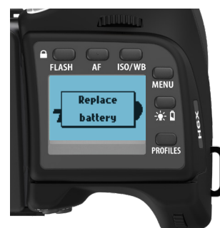
Exhausted battery warning
