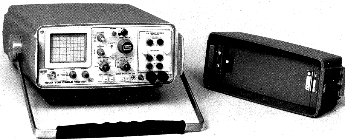
Fig. 2-1. 1503 Time Domain Reflectometer.
