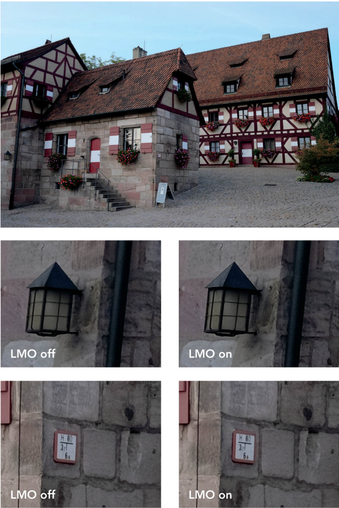
Fig. 43: This example illustrates how the Lens Modulation Optimizer (LMO) improves the edge and corner sharpness of Fujifilm's native XF and GF lenses. It was shot with an X-E2 and an XF23mmF1.4 R WR lens at f/8. Let's have a closer look at the lantern situated near the left edge of the scene: The two crops in the center row show the lantern with LMO OFF (left crop) and LMO ON (right crop). There's a small visible improvement in the version with the active LMO. However, if you compare crops of the sign taken from the center of the scene (bottom row), there's no visible difference between the versions with and without LMO. That's no surprise: Lenses achieve their maximum resolution around the image center, so the LMO's job is to only compensate the inevitable loss of resolution near the edges of the frame.
