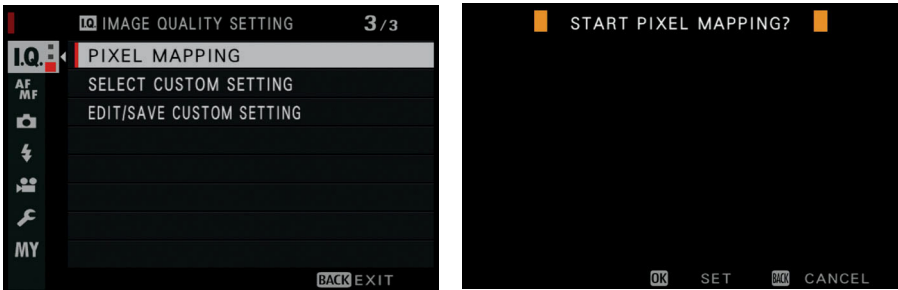
Fig. 31: Pixel mapping is a very useful function that is unjustly overlooked by many users. To avoid unpleasant pixel malfunctions in your images, it's best to apply it on a regular basis.
