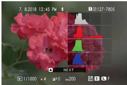
Fig. 93: This is the same RAW image, but this time processed with flat JPEG settings : Eterna film simulation, Shadow Tone -2, Highlight Tone -2, and Color -4. These settings reflect the flattest possible color profile that you can achieve in an X-H1, and there's now plenty of additional headroom in the shadows and highlights. Thanks to the much higher dynamic range of the flat JPEG, there's also no clipping of the red channel in the histogram. This flat JPEG reflects the dynamic range of the actual RAW file much better than the camera's default JPEG settings, and many RAW shooters use these or similar flat JPEG settings in concert with the RGB histogram because it makes it easier to determine the optimal exposure right at the sensor's saturation limit.
