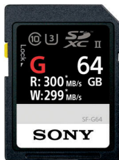
Fig. 23: For maximum UHS-II performance and compatibility, I recommend superfast Sony SF-G cards. Please note that these cards only make sense in cameras that explicitly support UHS-II, such as the X-T1, X-Pro2 (only slot 1), X-T2, X-H1, X-T3, and GFX. If your camera or card slot doesn't support UHS-II, you are better off using a fast UHS-I card like the SanDisk Extreme Pro 95 MB/s.
