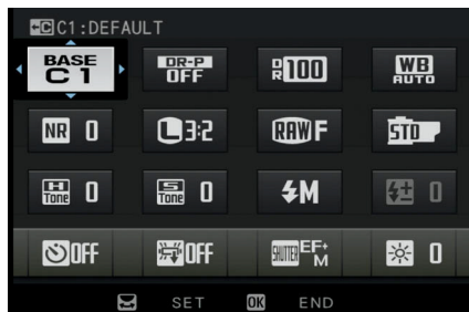
Fig. 76: The Quick menu page of my X-H1 and X-T3 isn't very different from the factory default setting. I always make sure that I can access the flash mode and the flash exposure compensation directly from this menu, and I like to have direct access to the shutter-type setting and flicker reduction. Since I don't need quick access to the COLOR and SHARPNESS items, I replaced them with the flash configuration items.
