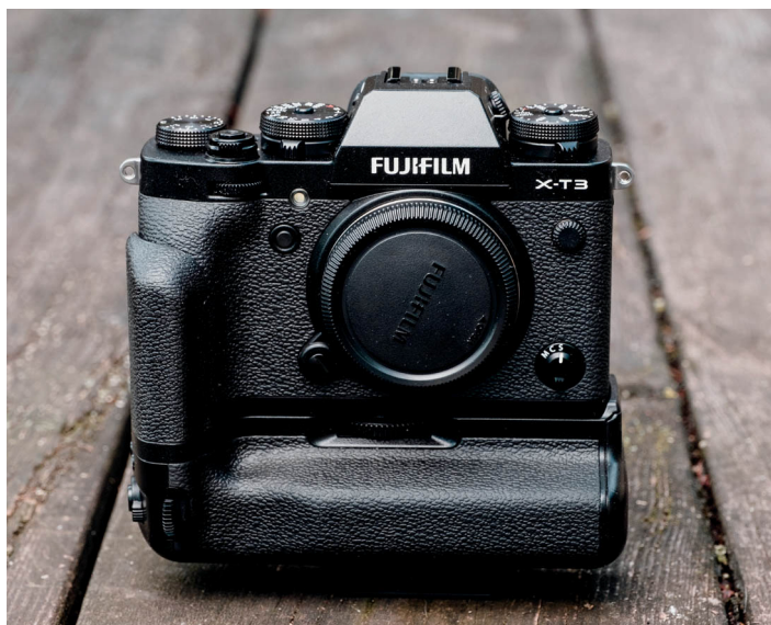
Fig. 11: The X-T3 is the original fourth-generation model in Fujifilm's system camera lineup. It's not hard to imagine that its back-side-illuminated 26 MP X-Trans CMOS 4 sensor and X-Processor 4 will also appear in future cameras, like a potential X-T30, X-E4, or X-Pro3.
