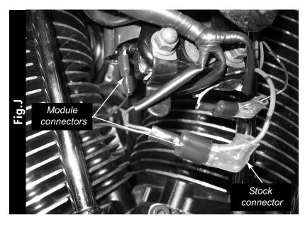
11 Unplug the RED/GREEN wire from the coils. Plug the RED colored wires from the Ignition Module in-line of the ignition coil and stock wiring harness (Fig. J)
