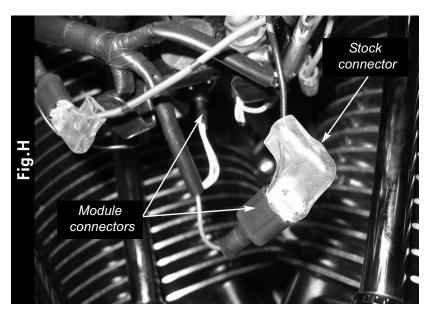
10 Unplug the BLACK wire from the coils. Plug the ORANGE colored wires from the Ignition Module inline of the ignition coil and stock wiring harness (Fig. H)
