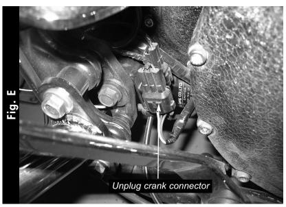
7 Locate the crank pickup coil connector on the front left hand side of the engine (Fig. E). Unplug this connector.
