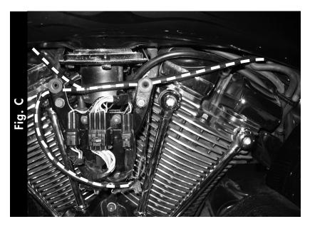
5 Continue routing the wiring harness along the left hand side of the engine (Fig. C).
