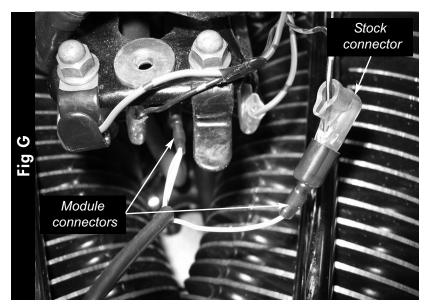
9 Unplug the BLACK/GREEN wire from the coils. Plug the YELLOW colored wires from the Ignition Module in-line of the ignition coil and stock wiring harness (Fig. G)
