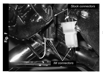
Plug the 3 pin connector from the Ignition Module in-line of the stock connectors (Fig. F).
