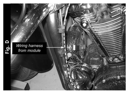
Route the wiring harness from the Ignition Module with the 3 pin connector along side the clutch cable down near the horn (Fig. D).
