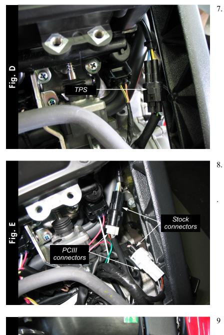
Locate the Throttle Position Sensor which is located on the right hand side of the throttle bodies. Unplug this connector (Fig. D).
