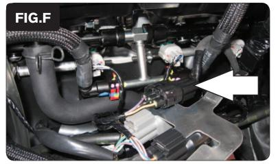
7 Connect the PCV harness in-line of the stock injectors and wiring harness (Fig. D).
