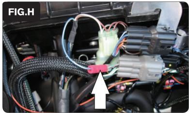
Attach the BLUE/WHT wire from the PCV to the GRN/RED wire of the stock gear position sensor (Fig. H).
