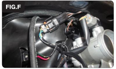
Plug the PCV wiring harness in-line of the fuel injector and the stock wiring harness (Fig. D).
