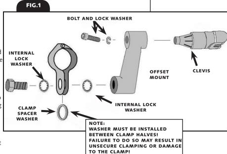
**STEP 7** Check the peg for proper location. If necessary, you can loosen the bolt that secures the clevis to the arm & adjust the peg mount and clamp position for maximum rider comfort. Tighten the bolt securely (refer to PIC.1.).
