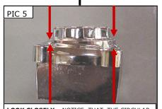
LOOK CLOSELY - NOTICE THAT THE CIRCULAR COGGED FACE OF THE SWING ARM MOUNT IS PLACED AT A TWO DEGREE ANGLE. PLACE THIS
