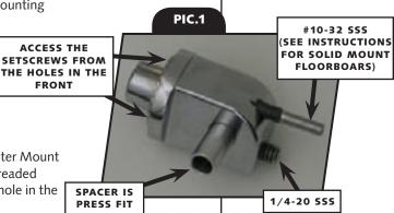
**STEP 7 FOR FOLDING FLOORBOARDS THAT REQUIRE A SOLID MOUNT.** Thread a #10-32 x 1 SSS into the upper hole in the Adapter mount as shown in <u>PIC.1</u>. Install flush with the back of the adapter. Ensure that the hex head end of the setscrew is threaded into the Adapter Mount so that it can be accessed through the hole in the splined face. See <u>PIC.1</u>.
