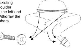
Align the Polished Stainless Steel Trim over the left and right holes and insert Stainless Steel Button Head Screws. Secure in place with Acorn Nut Shoulder Spacers.
