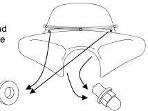
Align the Trim over the left and right holes and insert Button Head Screws.
