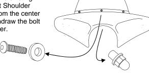
3. Align the Trim over the center hole and insert a Button Head Screw.
