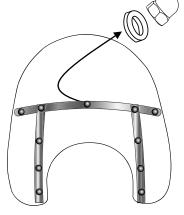
4. Align the pouch over the center hole and onto the exposed socket head cap screw. Screw in the socket head cap screw with the supplied allen wrench, and secure inside the pouch using the Short thumb nut (f)
