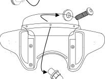
4. Align the pouch over the center hole and re-insert the Screw with Washer through the front of the fairing.
