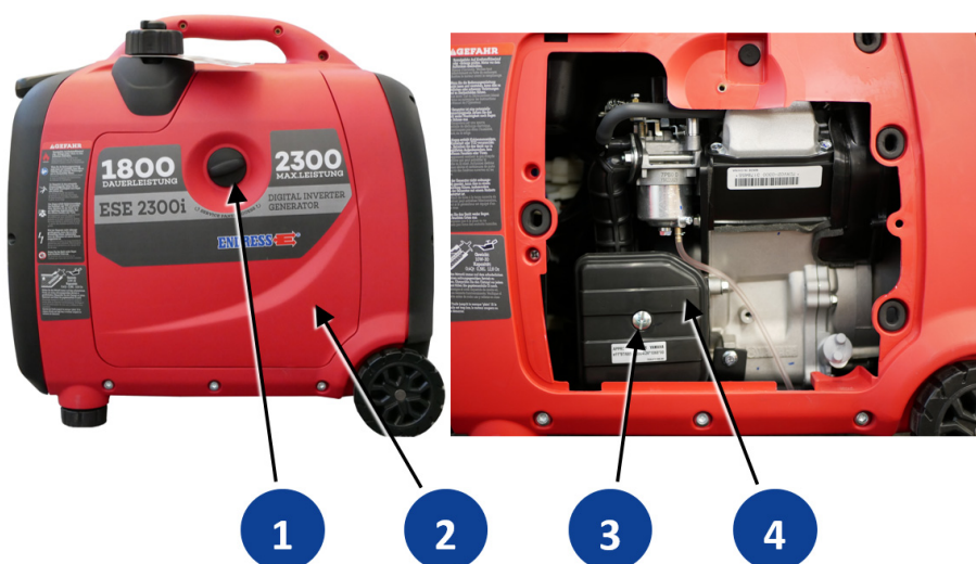
Fig. 8-4 Luftfilter bakom underhållsluckan (borttaget)
