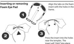
Press the insert into the holes above the nose piece. The insert will "click" into place.
