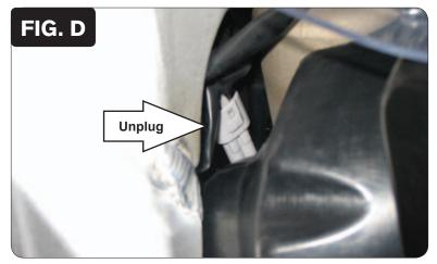
6 Unplug the Throttle Position Sensor harness (Fig. D). This connector is located behind the throttle body and is a WHITE 3 pin connector. It is best accessed from the right side of the bike.
