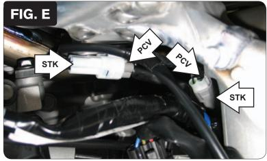
7 Plug the PCV harness in-line of the stock TPS and wiring harness (Fig. E).
