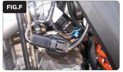
8 Plug the PCV in-line of the TPS and stock wiring harness (Fig. F).
