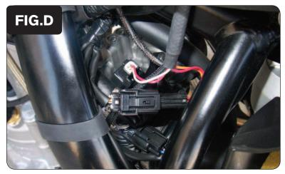
6 Plug the PCV in-line of the stock wiring harness and injector (Fig. D).
