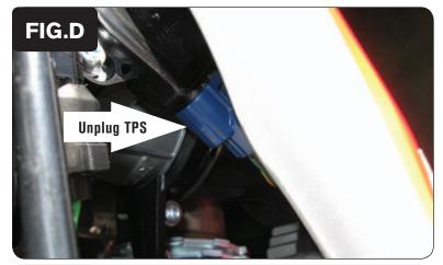
5 Unplug the Throttle Position Sensor harness (Fig. D). This connector is located on the left side of the throttle body to the inside of the frame.
