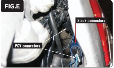
6 Plug the PCV harness in-line of the stock TPS and wiring harness (Fig. E)
