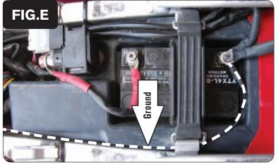
10 Attach the ground wire of the PCV to the negative side of the battery (Fig. E).
