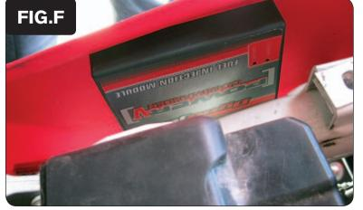
11 Using the supplied velcro attach the PCV to the inside of the left radiator shroud (Fig. F).
