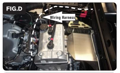
Route the remaining branch of the PCV wiring harness towards the rear, across the top of the fuel injector rail, and down the right side of the gear box (Fig. D).
