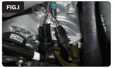
9 Plug the PCV wiring harness in-line of the fuel injectors and the stock wiring harness (Fig. G).
