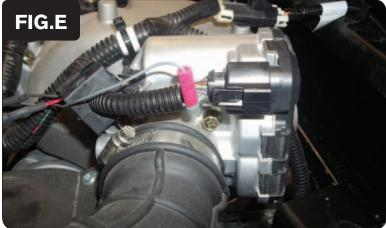
7 Using the supplied Posi-tap connect the GREY wire of the PCV to the GREEN wire of the stock Throttle Body Servo wiring harness (Fig. E).
