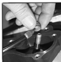
Install valve seals. Use protective sleeve on valve to protect seal during installation. Pre-lube seals with engine oil prior to installation
