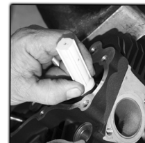
FEULING recommends the use a seal installer to prevent seal damage. Install spring, retainer & locks.
