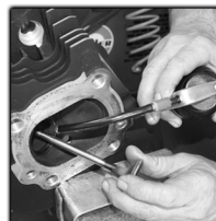
Pre-lube valves, install seat shims if needed, then install spring seats.
