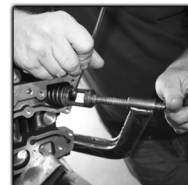
Remove original valve springs & hardware
