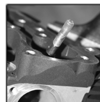
Install valve seals. Use protective sleeve on valve to protect seal during installation. Pre-lube seals with engine oil prior to installation
