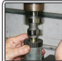
Press cam gears onto camshafts
