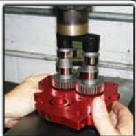
Line up timing marks, press in camshafts using lube and the proper tools
