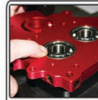
Verify bearings are flush with camplate
