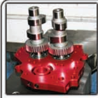
Line up timing marks, press in camshafts using lube and the proper tools
