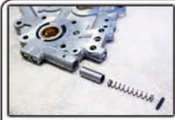
Inspect pressure relief valve
