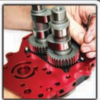
Install bearing retainer plate using loctite
