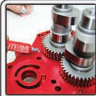
Install bearing retainer plate using loctite
