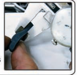
clay pistons and measure thickness of clay after cycling engine
