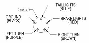
VIEWED FROM THE WIRE SCREW TERMINAL SIDE OF THE FEMALE TRAILER PLUG. TO INSURE CORRECT INDEXING ORIENT SLOT IN PLUG WITH RIB IN HOUSING.
