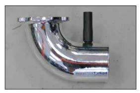
9. Cut the provided crankcase vent hose to a length of 1.75" and install onto the K&N® intake tube as shown.
