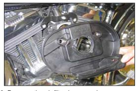
6. Remove the air filter base as shown.
