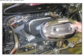
2. Remove the two air filter cover mounting bolts and then remove the cover from the vehicle as shown.
