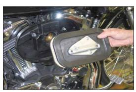
4. Remove the air filter as shown.
