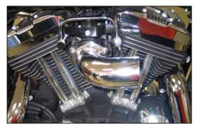
10. Install the K&N® intake tube onto the throttle body while attaching the vent hose to the vent tube and secure with the provided hardware.
