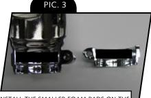
INSTALL THE SMALLER FOAM PADS ON THE INSIDE OF THE NECK COVER AND CLAMP
