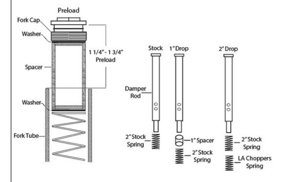
WARNING: Installing a lowering kit will decrease initial ground clearance. The motorcycle will be lower to the ground and care should be taken to avoid bottoming, especially over bumps or in turns. To maintain proper balanced geometry, the front and rear of the motorcycle should be lowered equally. Failure to properly install the lowering kit and operate the motorcycle after installation may result in serious injury or death to the rider.
