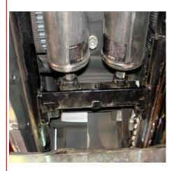
5. Assemble the new shock front hardware (bushing, cup washer and new lowering nut shown below). Use thread locker and install the shocks front hardware using a 3/4" wrench. Do not over tighten.
