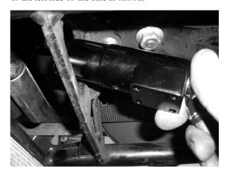
■ When mounting the RAP shock make sure the adjuster line is lined up towards the center of the bike and slightly up so it has as much clearance as possible going through the aforementioned frame window. Then mount the shock using the stock mounting bolts and washers, and tighten all shock mounting bolts to the proper torque specifications (see shop manual for specs).
