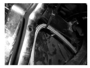
■ Route the line out the left side in front of the fender and above the lower belt-guard as illustrated.
