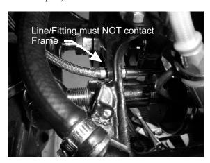
Route the line up and then to the left side of the bike. As you do so, you should tie off the line to the swingarm pivot as illustrated.
