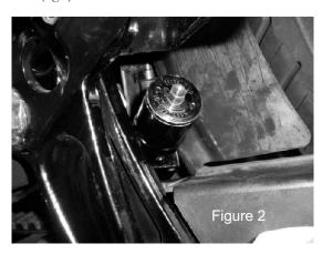
■ When mounting the RAP shock make sure the adjuster line is pointing to the right and slightly up as illustrated (fig.3).
