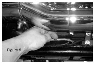
■ Route the line up and then to the left side of the bike. As you do so, make sure the line will not be pinched, kinked, or exposed to excessive heat and use the included zip-ties to secure it in place. Route the line out the left side in front of the fender and above the lower belt-guard (fig.6).
