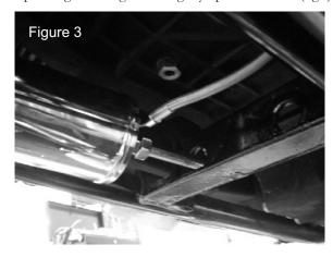
■ Then install shocks as you would a stock unit, following an authorized shop manual - noting to route the adjuster line in a sweeping arc above the right non-RAP shock and towards the rear of the bike. With the non-flanged nut spun all the way onto the stud, the stock ride height is achieved (ride height adjustment will be addressed later).
