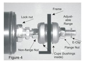
Mount the rear eyes of the shocks using the stock bolts and washers, and tighten all shock mounting hardware to the proper torque specifications (see shop manual for specs). Route the adjuster line in a seeping arc above the right shock and toward the rear (fig.5).
