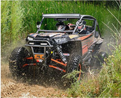
A 2014 Polaris RZR XP 1000 has 16" of travel out front, 18" in the rear, and 13.5 inches of ground clearance to tackle almost any terrain
