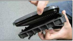
12. Remove the stock filter and Install the new  $K\&N^{\ensuremath{\mathbb{R}}}$  filter.
