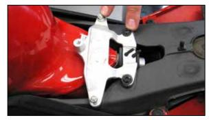
2. Remove the hardware shown and remove fuel tank bracket.
