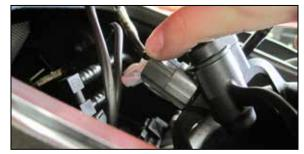
8. Disconnect front and rear injector connectors.
