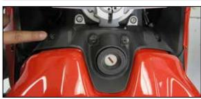
3. Remove the four allen screws shown
