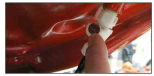
7. Disconnect fuel line under fuel tank. WARNING: Some fuel will spill out; have a rag ready to absorb any spillage.
