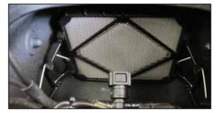
and remove ignition cover above fuel tank.
