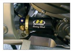
Another way to mount the reservoir is with hose clamps and rubber blocks. The reservoir is then attached to one of the frame tubes. The picture on the left shows an example.
