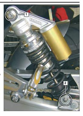
Place the shock in the motorcycle; place the top bolt (1). Lift the rear wheel up in order to place the bottom bolt (2) Tighten the nuts. Place (when necessary) the remote reservoir on its place and (when necessary) the hydraulic preload adjuster knob in place.
