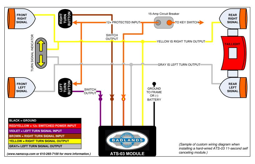
The wire colors in the drawing are used for reference only based on the colors we use on our module. When installing the hardwired ATS-03 on a factory model, be sure to consult your bikes service manual for exact wiring diagrams and color descriptions to achieve proper installation.
