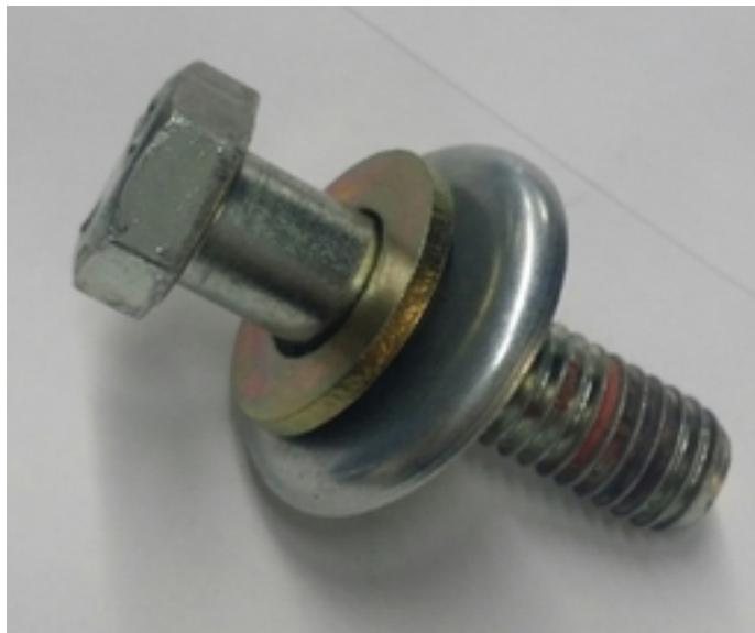
3. Install a supplied 1/2" flat washer on each stock mounting bolt between the bolt head and the bottom cup washer. This is to space the stock bolt down ever so slightly so that the bolt does not protrude into the area where your handlebar mounts.
