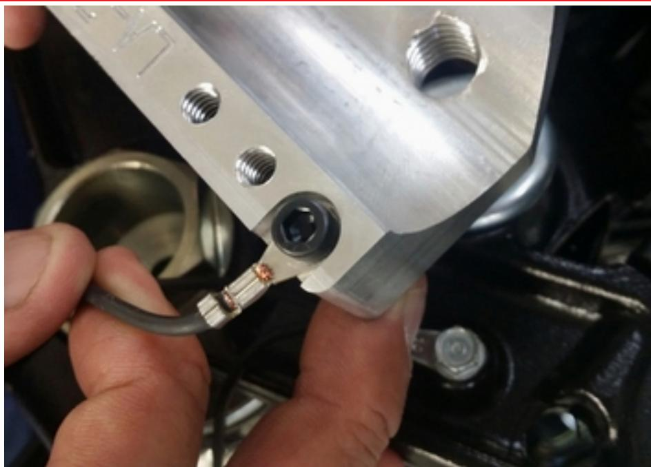
Next secure the ground wire with supplied 10-32" bolt. You must do this before installing the top clamp.
