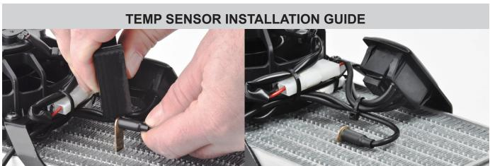
Carefully insert the temperature probe into fins of radiator.
