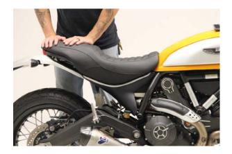
3. Lower the seat onto the rear fender, align the pin with the latch on the fender, and press down firmly until a click is heard, signifying the seat is latched. Ensure this connection is secure before riding the motorcycle.
