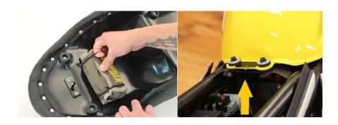
2. Insert the front tab of the Mustang seat into the mount behind the fuel tank.
