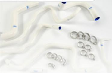
There are many substances that will remove dirt and grime from engine components, but not that many are suitable for silicone. The best cleaning product is a simple solution of soapy water. **Do not** use petroleum based products under any circumstances.
