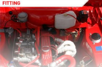
Pipe work should be matched to the hose to ensure a good interference fit without overstretching. Hoses must never be distorted when fitted, if the hose is stretched into position it is more likely to fail. Hoses when clamped in place should be clamped just behind the formed bead with at least 10mm of hose beyond the clip. (Hose Fitting Guide)
