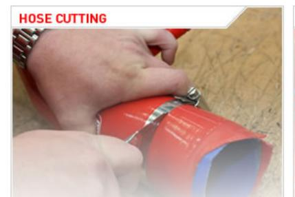
To cut silicone hose use a new 'snap off blade in your knife. Tighten a jubilee clip around the hose without deforming the hose and use the edge of the clip as a guide for the knife blade. Stop near the worm drive section as the band here is uneven. Then take off the clip and slice through the remainder with the hose resting firmly on a flat service.
