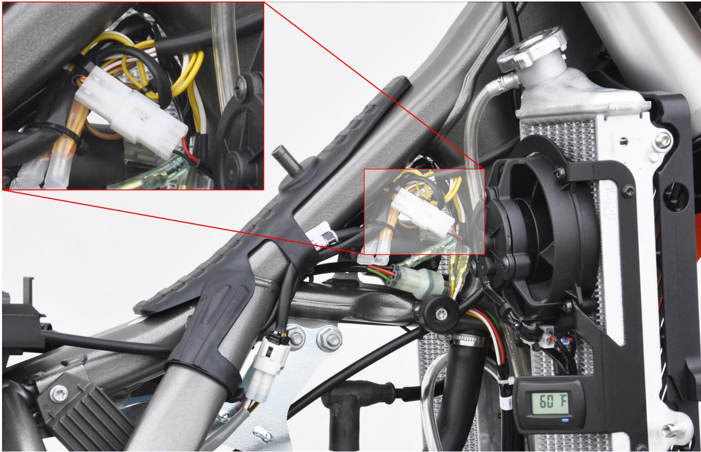
7.) Connect fan kit to bike power. If the motorcycle came from KTM/HUSQVARNA with the fan harness then the Trail Tech fan kit will plug directly into the factory connector. This is located just to the left of the radiator in the wiring above the motor (*See above photo*). If the motorcycle did not come with a factory harness, then install the provided power lead for the fan kit. Connect the ring terminals directly to the machine's battery (*Black to negative, red to positive*).
