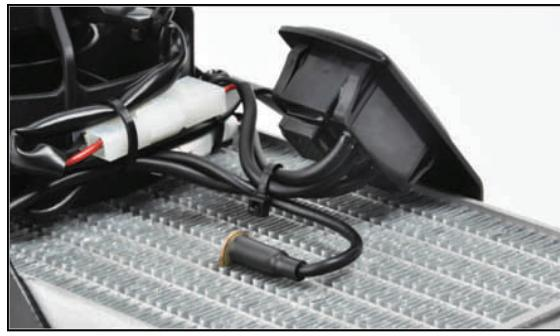
**TIP:** To compensate for the influence of ambient air passing across the sensor, apply thermal grease (included in kit) into the gap between the fins of the radiator where the sensor will be installed. It is important to place the grease only in the gap. Grease on the surface of the radiator will attract dirt and reduce function.
