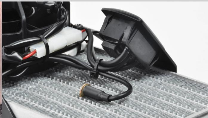
5.) Carefully insert the temperature probe into fins of radiator.
