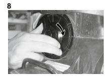
NOTICE Ensure air filter flange is properly inserted into the hole at the other end of the air filter box.
