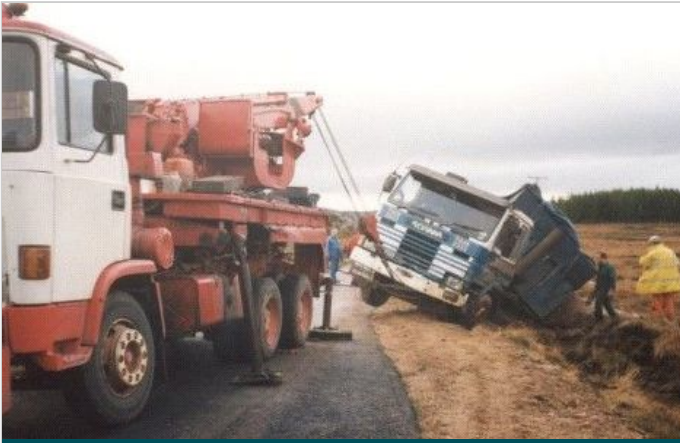
The heavy lift recovery vehicle in action
