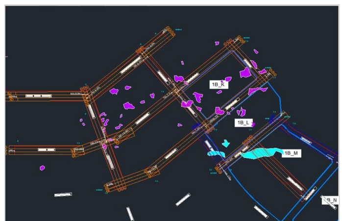
Void spanning mitigation on estate roads
