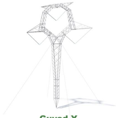
Guyed Y Lattice Tower
