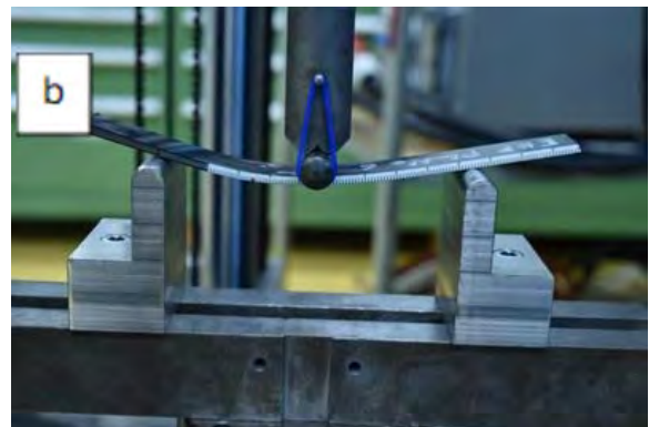
Figure 1b: End-Notched Flexure (ENF) test specimen
