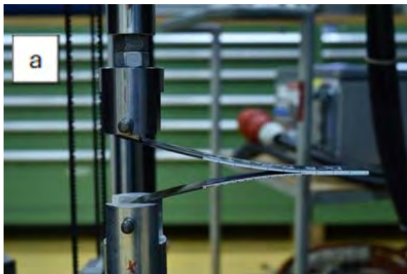
Figure 1a: Double Cantilever Beam (DCB) test specimen
