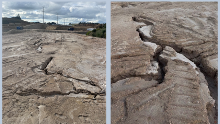
Photos: examples of extensive erosion on Tauriko pumice soils, 15mm of rain, 30m slope length with less than a 3% grade.
