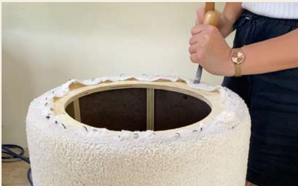
Lifting staples with tack hammer and staple lifter, working away from my body
