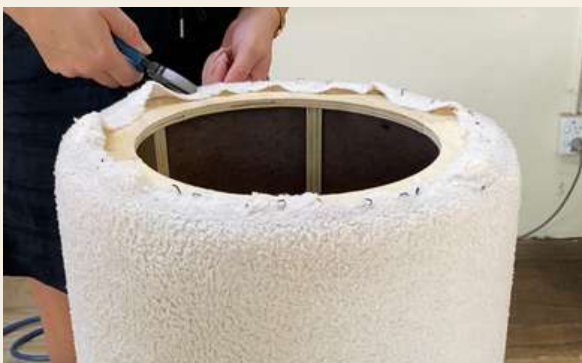
Removing staples completely using spring loaded pliers.
