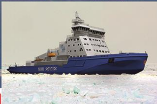
The new icebreaker of the Finnish Transport Agency features the highest technology and has been designed especially for the demanding icebreaking operations in the Baltic Sea. She will use both diesel and LNG as its fuel, which diminishes her emissions and operating costs. She will also be equipped for oil spill response operations and emergency towing missions. Delivery 2016.
