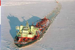
Double Acting Ship (DAS™) MT "Tempera" in the Gulf of Finland during in severe ice winter 2003.
