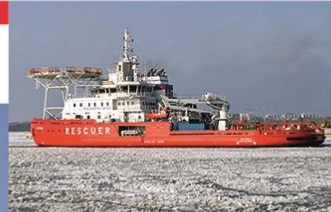
The world's first oblique icebreaking emergency and rescue vessel "Baltika" delivered in 2014 from Arctech Helsinki Shipyard can break sideways 50 m wide channel in 0.6 m thick ice.
