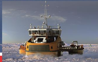
Multipurpose Harbour Icebreaker Trimaran Tug is one of the latest innovations in icebreaking. The concept was able to create a channel twice the width of a channel of a traditional icebreaker, but with the same propulsion power!
