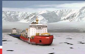
Aker Arctic was a member in the team led by local STX Canada Marine that have been awarded the contract to design the new polar icebreaker "John G. Diefenbaker" for the Canadian Coast Guard. The polar icebreaker will be designed to accommodate 100 personnel with space for 25 additional people and have the ability to break through 2.5 m of ice at 3 knots.
